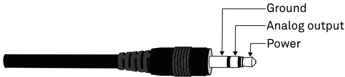
Figure 1 Stereo plug connector
